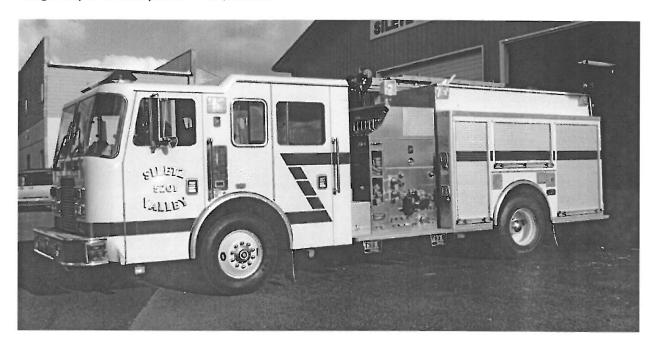
This engine has been re-assigned at Station II as our second out fire engine to respond to all fires and utilized often for training and other local activites. Engine was stocked with new 4" hose (upgraded from 3") in 2014, numerous adapters and fittings, a new hose bed cover to protect the hose from the elements, as well as a handful of hand tools and necessary supplies. It is equipped with six (6) Self Contained Breathing Appartus (SCBA) and seating for 6.
