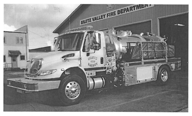
This tender utilizes the newest technology in water transfer vehicles. The vacuum pump creates a vacuum that fills and empties this vehicle in less than two minutes.
